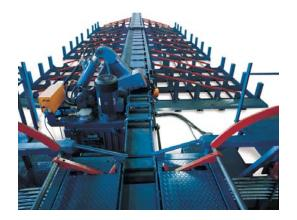
The system integrates the RSM 50.300 shear with conveyor width of 320mm. Option of single side or double side cut steel storage. The gauge table discharges the cut steel with pneumatically operated tilt action in both directions into 3, 4 or 5 storage bins per side. The conveyor rollers are 45 degree gravity coned to prevent steel running off the conveyor rollers.
